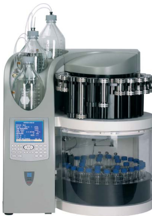
Figure 9 Thermo Scientific™ Dionex™ ASE system 350 apparatus from Dionex. Up to 24 samples (1–100 g each) may be sequentially extracted in 1, 5, 10, 22, 34, 66, and 100 mL cell sizes. (Source: Reproduced with permission of Thermo Fisher Scientific Inc.)
