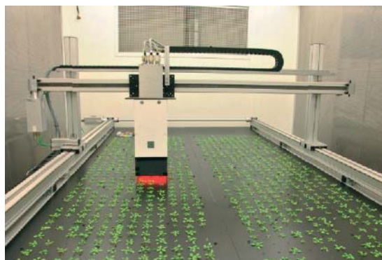
Figure 10 A robotic high throughput system for imaging small plants, such as Arabidopsis thaliana , using visible light, near-infrared, and chlorophyll fluorescence. In this design, the camera is attached to a robotic x-y movement system that allows the imaging head (which includes LEDs to supply the measuring light for the various imaging channels, and a camera with a filter wheel for wavelength-specific imaging) to be moved to a randomly chosen group of plants. The plants are grown hydroponically in individual rock-wool blocks that are securely fixed beneath a black plastic cover plate that also provides a good background for the plant images. The plants are watered using an ebb and flood system and the complete system is installed in a growth cabinet for good environmental control (Harbinson et al. , 2012). (Source: Reprinted from Curr. Opin. Biotech. , 23, Harbinson J., Prinzenberg A.E., Kruijer W., and Aarts M.G., High throughput screening with chlorophyll fluorescence imaging and its use in crop improvement, 221–226, Copyright 2012, with permission from Elsevier.)
