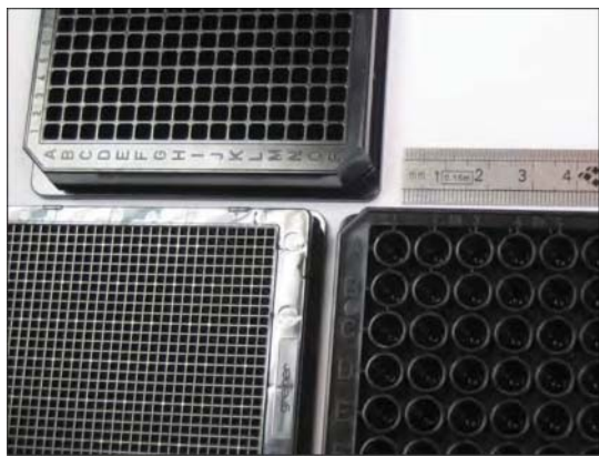
Figure 6 The 96, 384, and 1536 plate formats. In the 96-well format (right), each well occupies approximately a 50 \text{mm}^2 surface enabling automated and manual experiments. This is important for bioassay development, which can be made in the same format as in HTS. In the 384-well format, well surface is close to 12 \text{mm}^2 and still enables the two types of experiments. In the 1536-well format, well surface is close to 3 \text{mm}^2 and only very simple experiments could be run manually on a small part of the plate.
