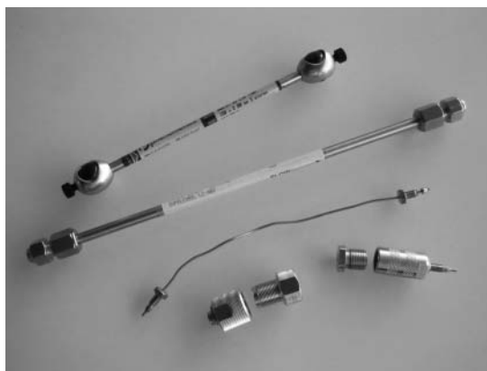
Figure 4 The heart of any HPLC instrument. From top to down: two columns of different length and with different end fittings, a connecting capillary, another type of end fitting, and a precolumn holder.
