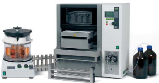
Figure 10 E-916 SpeedExtractor device from BUCHI Labortechnik AG. Up to six samples can be simultaneously extracted in 10, 20, and 40 mL cells. The collection vessels (60, 220, and 240 mL) can be transferred directly to the parallel evaporator Multivapor™ P-6. (Source: Reproduced by permission of BUCHI Labortechnik AG.)
