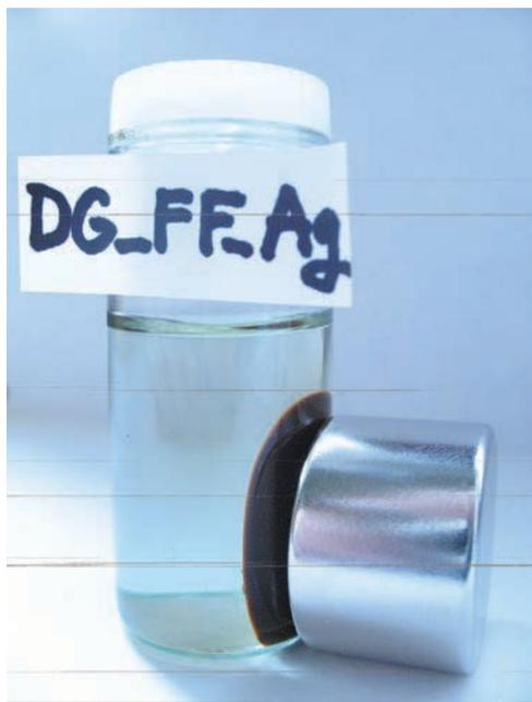
**Fig. 5.9.** Illustration of ferrofluid modified bionanocomposite behaviour in external magnetic field. This figure is reproduced from Schröfel (2012) with permission of the author.
