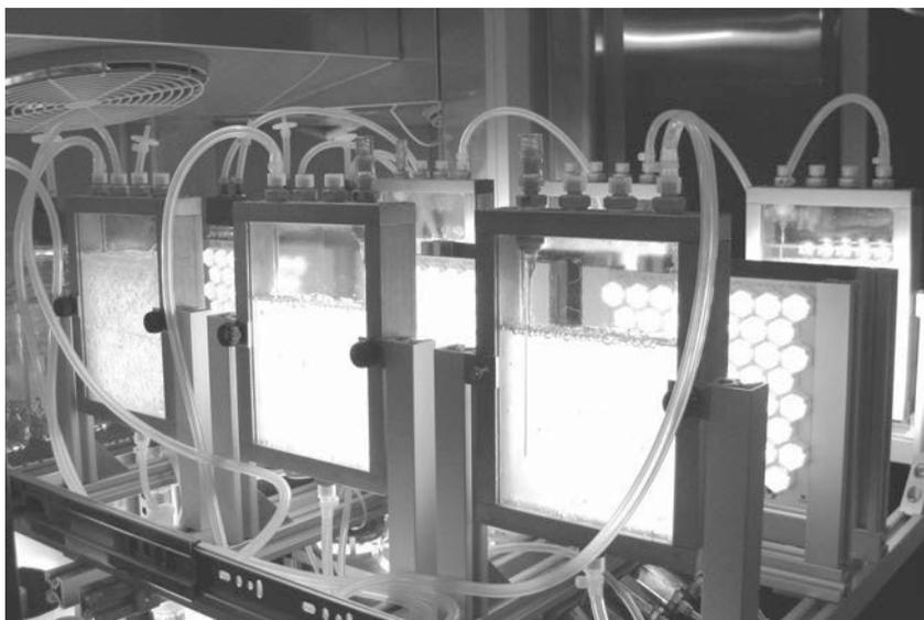
**Fig. 13.2.** A system of mini flat-plate photobioreactors with LED illumination used for the cultivation of *Emiliania huxleyi* and *Pleurochrysis carterae* in the Institute of Bioprocess Engineering, Karlsruhe Institute of Technology, Germany.
