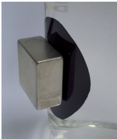
Figure 10.2. Ferrimagnetic Pd/nano-magnetite particles are easily separated in everyday laboratory life by permanent magnets.
