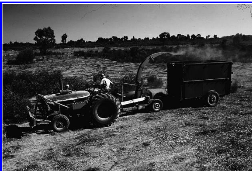
FIGURE 5.20 Harvesting blue mallee with distillation container.
