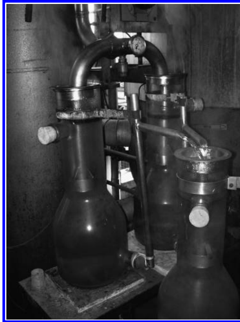
FIGURE 5.19 Orris distillation, Florentine ask at nearly 98°C.
