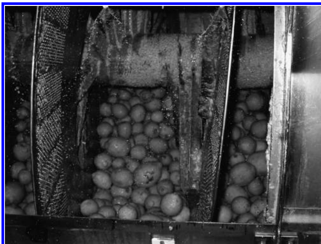
FIGURE 5.5 “Pellatrici” method. The spiked Archimedes screw with lemons, washed with water.
