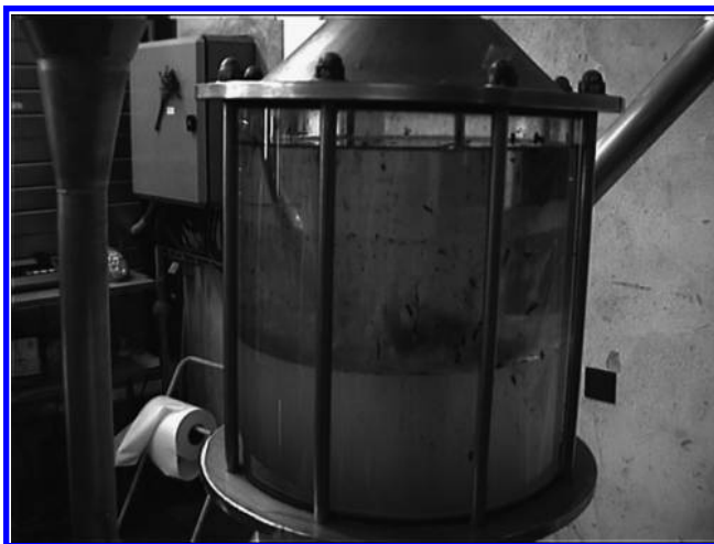
FIGURE 5.18 Oil and muddy water in the Florentine ask.
