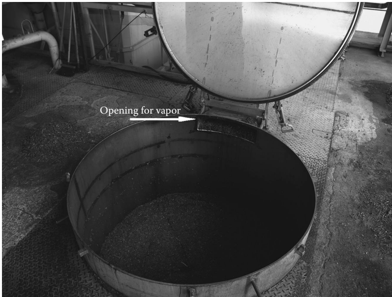
FIGURE 5.12 Open kettle with opening for vapor and oil.
