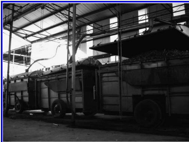
FIGURE 5.21 A battery of containers to be distilled, one opened to show the biomass.
