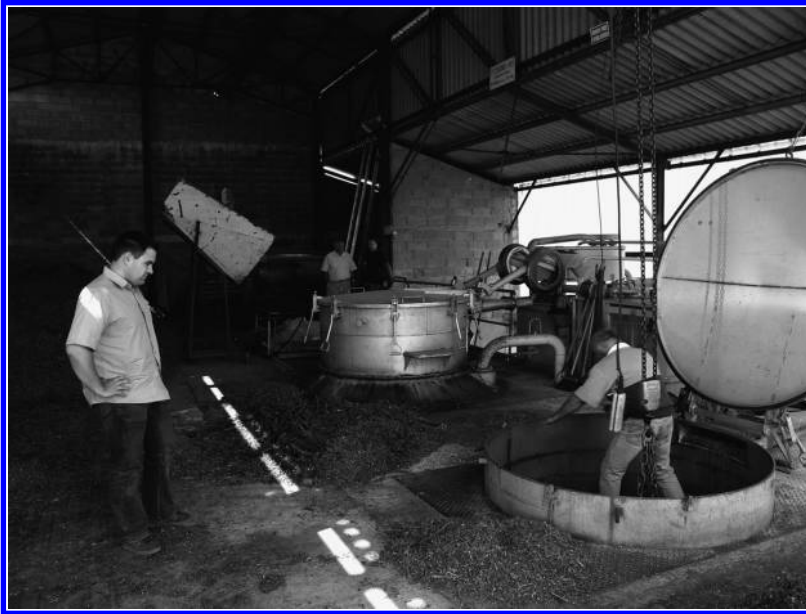
FIGURE 5.14 Loading a kettle and pressing by concreted tractor wheel.
