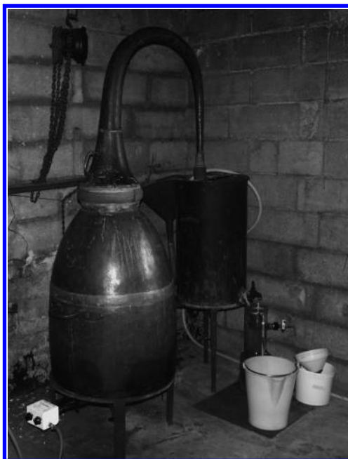
FIGURE 5.9 Old distillation apparatus modernized by electric heating.
